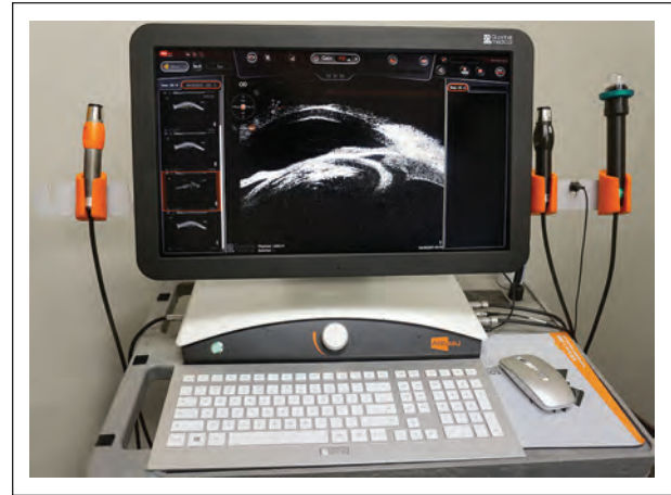
Figure 1. This figure shows a typical ultrasound instrument with ultrasound transducers (Quantel Absolu, Bozeman, MT) used to image ocular structures. On the left side of the monitor, there is a 20 MHz transducer used for posterior segment imaging. On the right side of the monitor, there is a 15 MHz transducer (left) also used for posterior segment imaging and a 50 MHz transducer with a green sleeved cover filled with solution used for anterior segment imaging (right).
